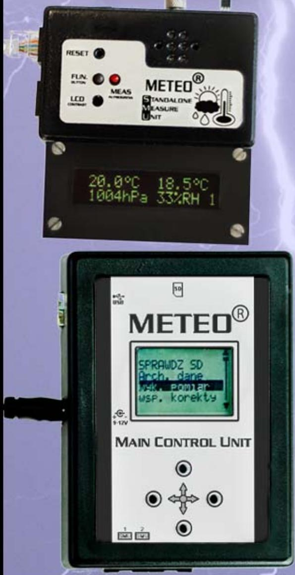
The goal of this project was to create a system meter of environment parameters in the test laboratory. The system was to provide measurements of temperature, humidity and pressure, dispose of non-volatile memory for measurements (min.10000), ensure co-operation with the PC.
